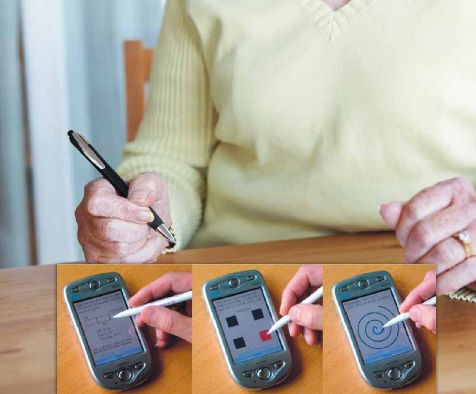
Figure 1. A photograph of the telemetry test battery. The test battery consisted of a patient diary section for collecting self-assessments of symptoms and a motor test section (tapping and spirography) for collecting objective measures of upper limb motor function.
